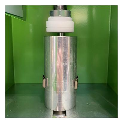
Push the can with the filling cylinder into the device until the side clamps engage, positioning the filling cylinder directly beneath the piston.
